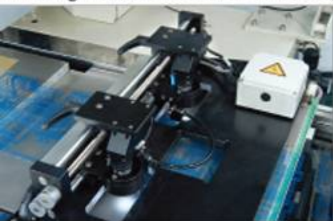
CCD雙鏡頭視覺系統 Double lens CCD visual positioning control system features high accuracy.
